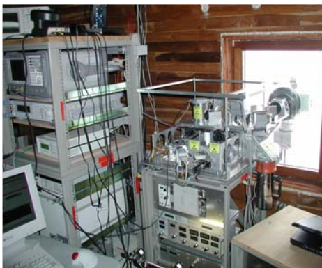
The 268 – 280 GHz-Radiometer installed inside the MARS station
