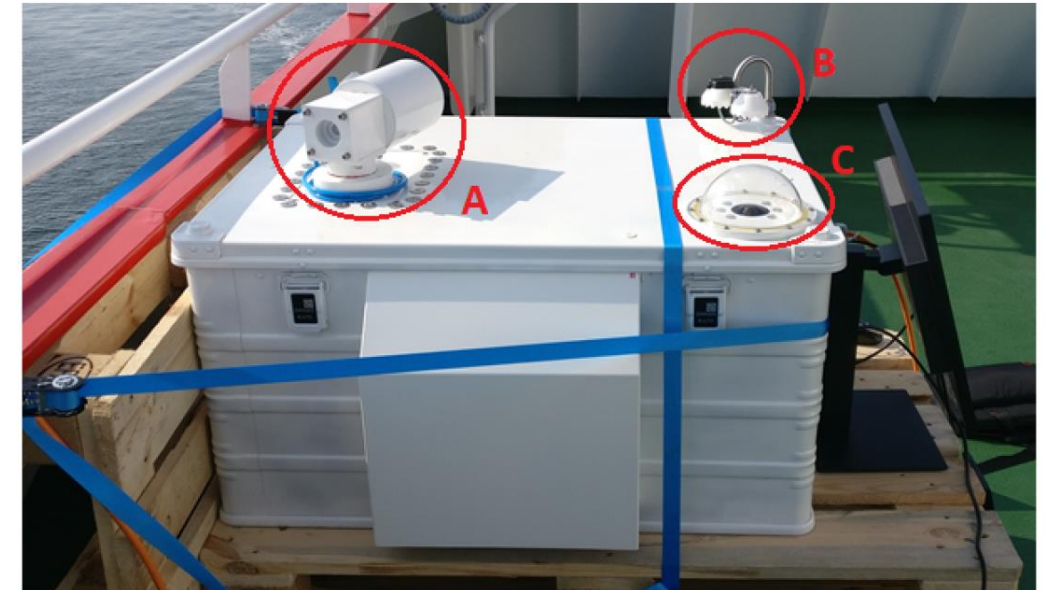
Ship-going variant of EM27/Sun Fourier Transform Spektrometer (Bruker Optics) with custom-built sun-tracker und sealed housing.
