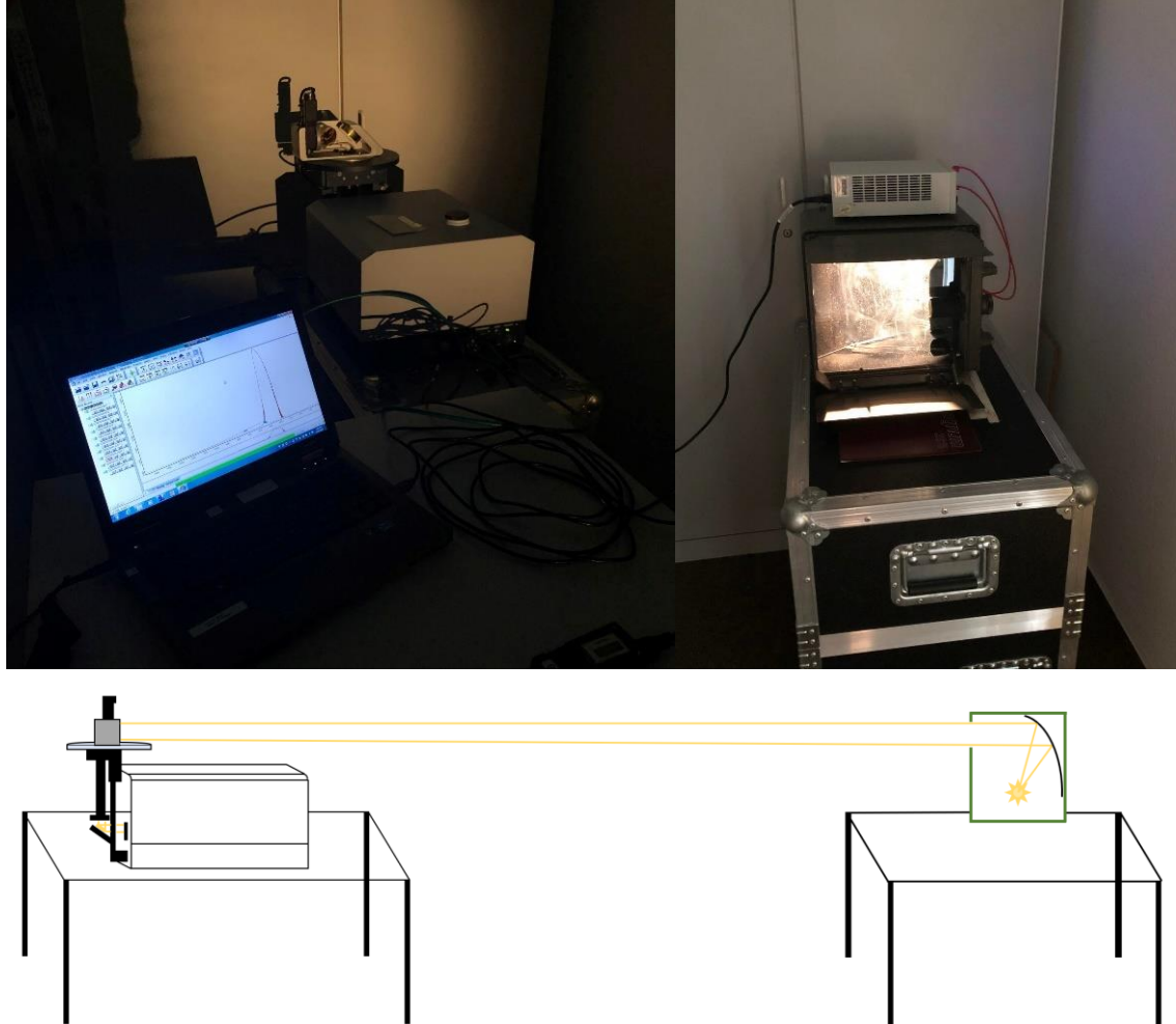
Figure 4.1. The top right and left panels are pictures of the spectrometer and light source taken during the measurement. The bottom panel is the schematic drawing of the setup where CO 2 concentrations were measured in between the optical pathlength.
