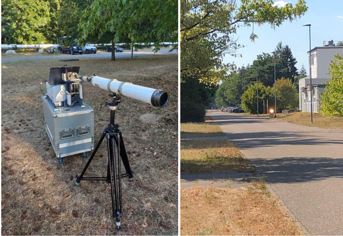
Figure 4.8. The optical setup with a telescope system in between the spectrometer (left) and the light source (right) for CO 2 open-path measurement.
