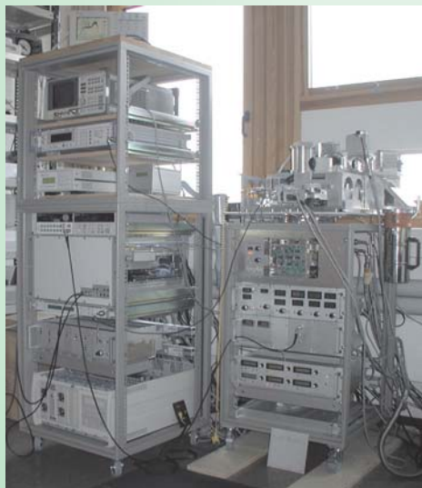
MIRA2 with the Acousto-Optical Spectrometer (AOS) and PC control rack (left)
