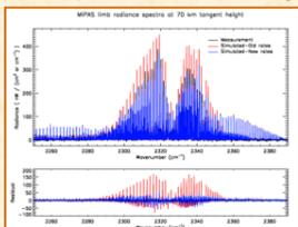
MIPAS limb spectra near 4.3 μm measured and calculated with old and new collisional rate constants for the relaxation of the CO<sub>2</sub> 2.7 μm levels (02<sup>0</sup><sub>1</sub>, 02<sup>2</sup><sub>1</sub>, 10<sup>0</sup><sub>1</sub>) (HITRAN: 23, 24, 25).
