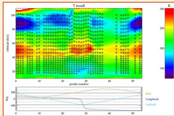
Temperatures retrieved from MIPAS spectra in its upper atmosphere mode, orbit #1750 on 1 Jul 2002. Scans 0–23, 53, 54 are taken in the daytime at 85°N–60°S; 25–50 cover 85°S–60°N in the nightside. The retrieved data shows the typical temperature structures of solstice conditions:
