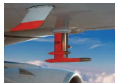
Gas inlet for the CARIBIC project installed on a commercial Airbus A340-600
