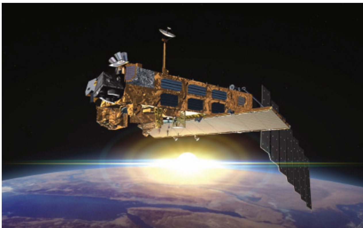
The European ENVISAT satellite (in orbit since 2002) carries three instruments for atmospheric research: MIPAS, GOMOS and SCIAMACHY
